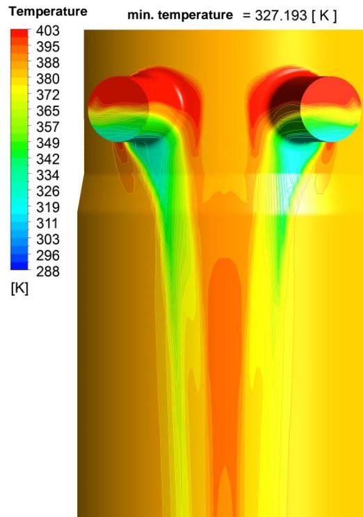
Fig. 5: Cold water streaks in the downcomer
