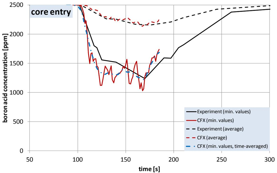
Fig. 4: Boron concentration at the core entry (ROCOM experiment PKL III E2.3)
