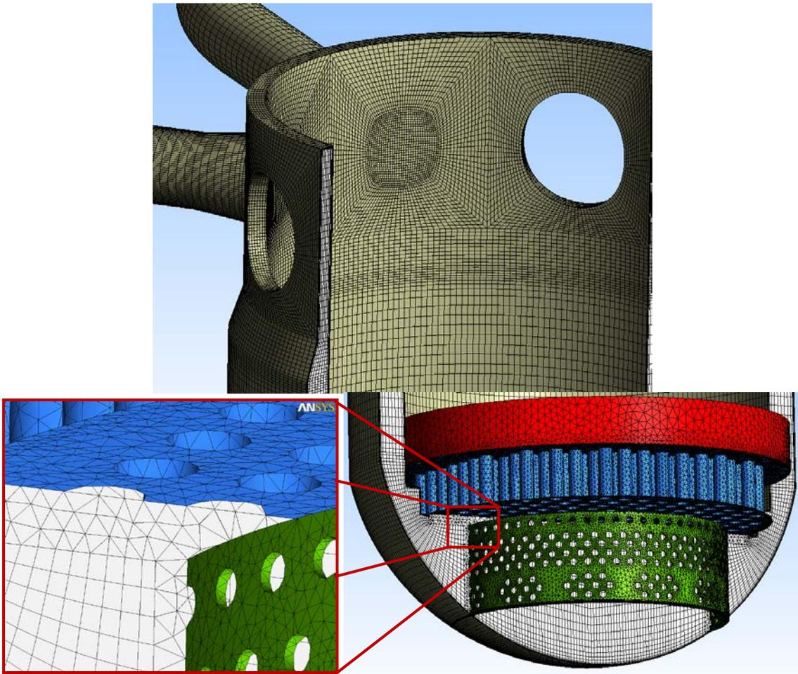
Fig. 3: Snapshots of the hybrid mesh
