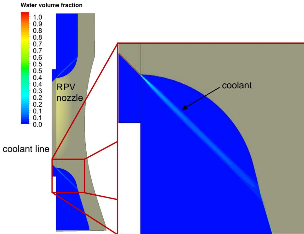
Fig. 8: Side view of the RPV inlet nozzle and
