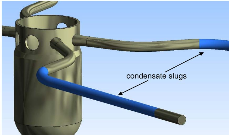
Fig. 1: CFD model of the ROCOM test facility
