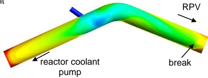
Fig. 7: Temperature distribution (pipe bottom)
