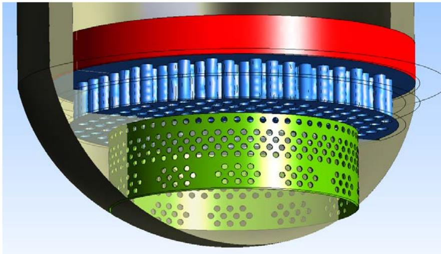
Fig. 2: Lower plenum with perforated drum
