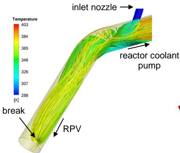
Fig. 6: Streamlines of emergency coolant
