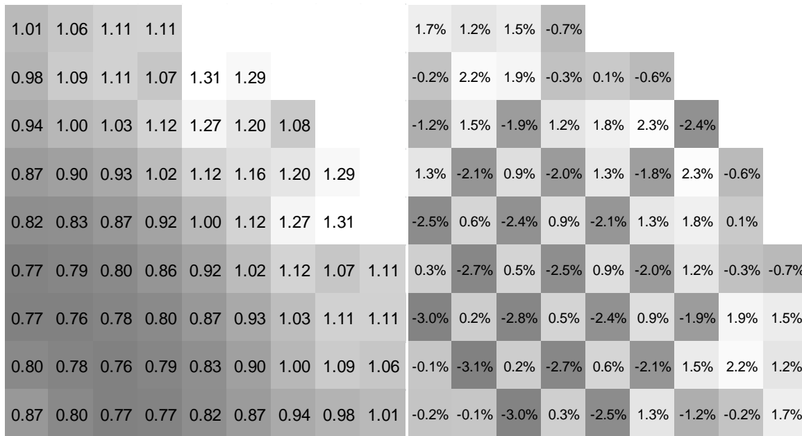
Figure 6 - Power distribution in the UOX core: KENO V.a results (left) and relative differences between KENO V.a and QUABOX/CUBBOX results (right). Quarter symmetry is displayed.
