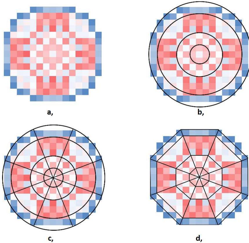
**Figure 2, Nodalization of the core, asymmetric case. Current and new method (colors indicate the power distribution compared to the average power of a fuel element)**
