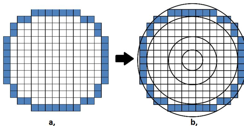
Figure 1, Nodalization of the core, current method. Symmetric case
