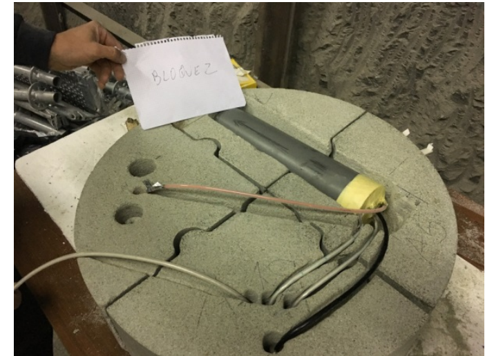
Wireless transmitter connected to new psychrometers, conventional pore pressure and relative humidity sensors
