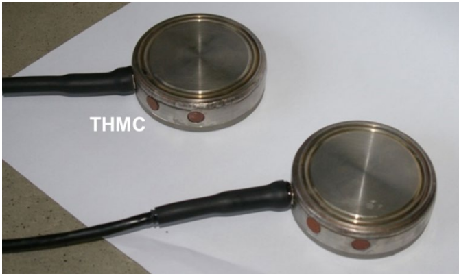
THMC smart sensor (measures total pressure, pore pressure, temperature and relative humidity)
