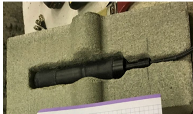
Chemical sensor based on measurements of potential difference between an ion-selective electrode and a reference electrode (measuring electrodes pH, Eh and Cl-)
